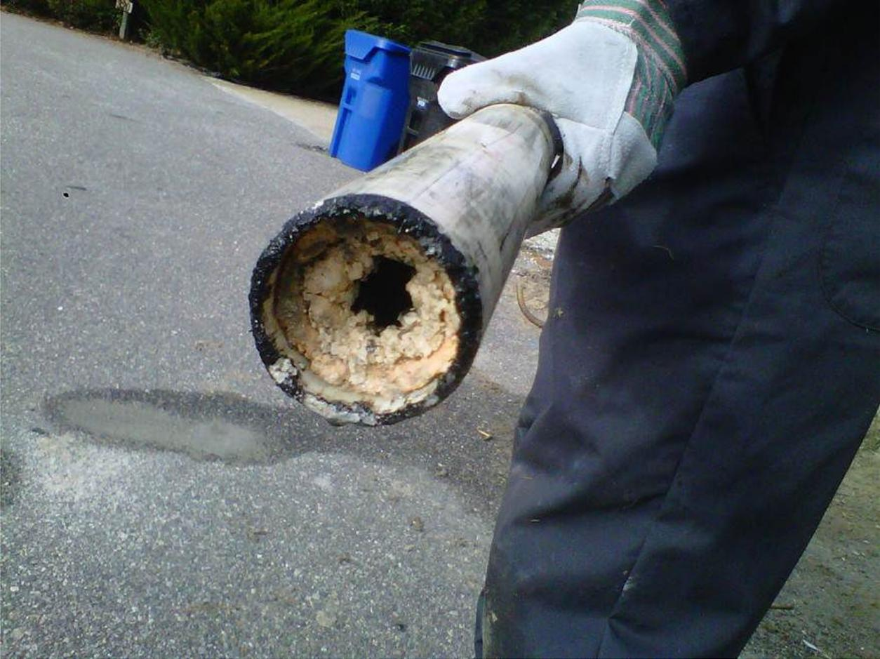
Shown below, grease is building up in gravity system sewer main pipes.
